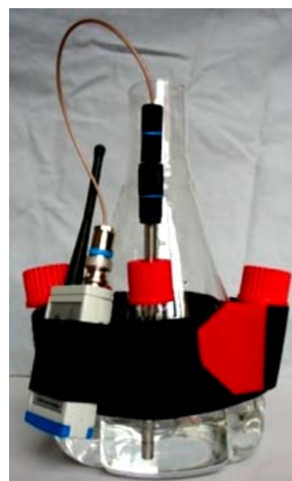
Fig. 3: SENBIT Flask equipped with a pO 2 electrode
