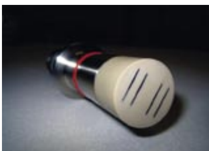
Photo 1: Flush electrode probe developed initially for cell culture and brewing
